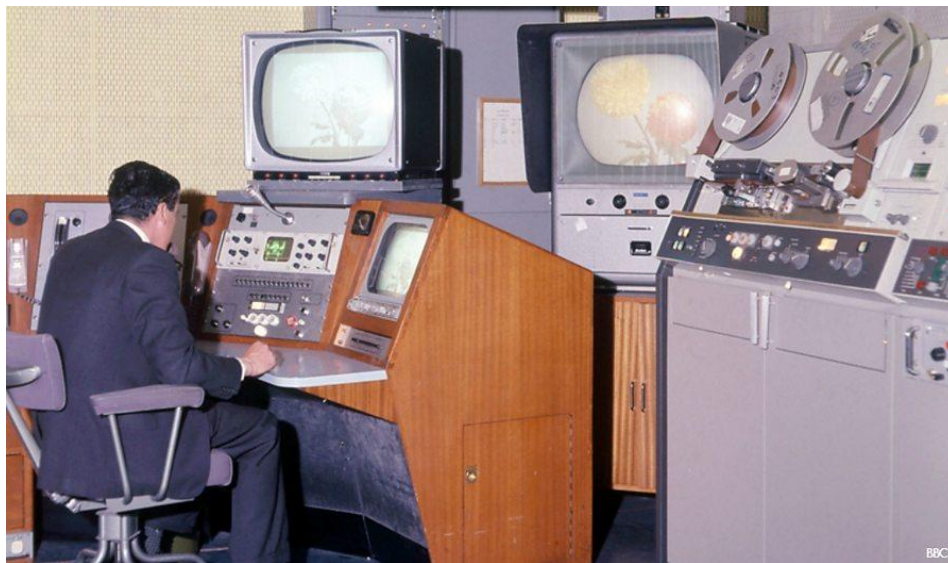
Plate 4a. Reel-to-reel video tape recorder (right of the picture) in BBC video suite circa 1968.
